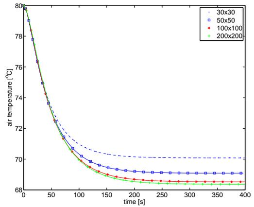
Figure 7: Outlet value of the air humidity over the time for ROWDA3 method with different grid sizes.
