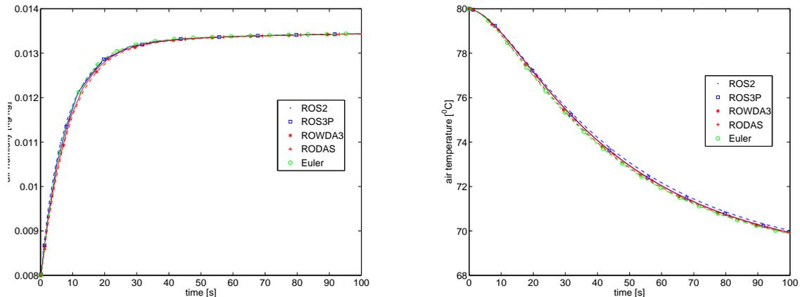
Figure 5: Outlet value of the air humidity and air temperature over the time for different time stepping methods.
