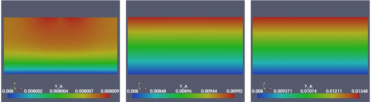
Figure 4: Solution of the air humidity at time  $t = 0.1 s$ ,  $4.03 s$ ,  $400 s$ .
