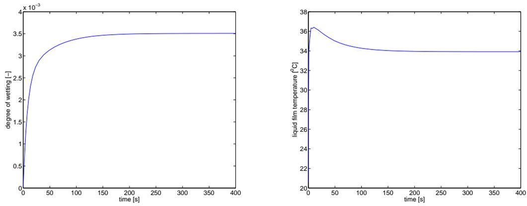
Figure 2: Outlet value of the degree of wetting and liquid film temperature over the time.
