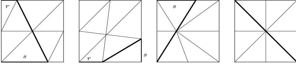
Figure 5: Different types of cut patches. From left to right: *A*, *B*, *C* and *D*. The subdivision can be anisotropic with  $r, s \in (0, 1)$  arbitrary.
