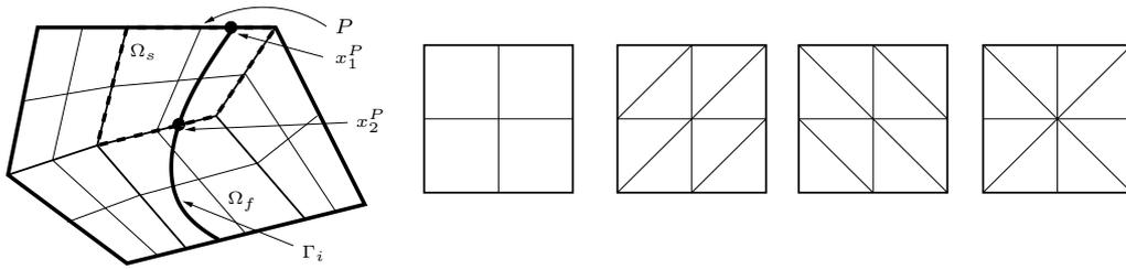
Figure 4: Left: triangulation  $\Omega_h$  with interface  $\Gamma_i$ . Patch  $P$  is cut by  $\Gamma_i$  at  $x_1^P$  and  $x_2^P$ . Right: subdivision of reference patches  $\hat{P}_1, \dots, \hat{P}_4$  into four quadrilaterals or eight triangles.
