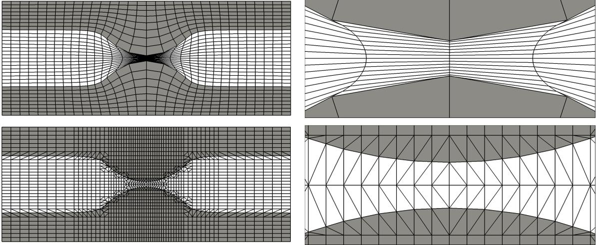
Figure 7: Biharmonic deformation (on top) close to break-down at  $\tau = 109.3$  days and zoom-in at right. On the bottom the corresponding meshes at the same time instance  $\tau = 109.3$  days for the fully Eulerian approach are provided.
