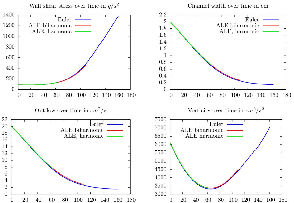
Figure 6: Long-Scale Problem: Course of different functionals over time (in days). *Top left:* Averaged wall stress  $\sigma_{WS}$  in  $g/s^2$ . *Top right:* Channel width in cm. *Bottom left:* Outflow  $v \cdot \vec{n}$  over  $\Gamma_{f,out}$  in  $cm^2/s$ . *Bottom right:* Averaged vorticity in  $cm^2/s^2$ .
