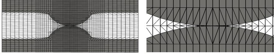
Figure 9: Example 8.1.2: Fully Eulerian deformation when the channel is completely closed at  $\tau = 55.8$  days.
