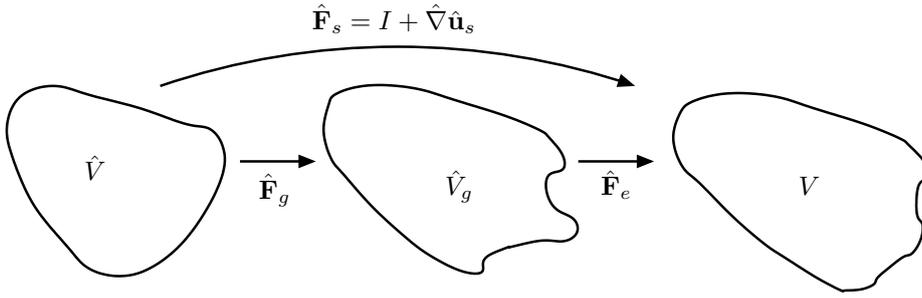
Figure 2: Volume elements  $\hat{V}$ ,  $\hat{V}_g$ ,  $V$  and deformation gradients linking them.  $\hat{V}$  denotes the stress-free Lagrangian configuration,  $\hat{V}_g$  an intermediate (non-physical) configuration after growth and  $V$  the current volume element.
