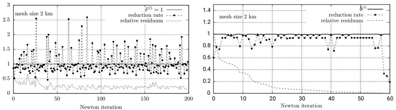
Figure 1: Sea ice simulation on a mesh of 2km mesh size (which is considered as very accurate within the community). Left: simulation with standard Newton with line-search. No convergence is observed. Right: the operator related damped Newton gives convergence. It is observed that the adaptive control required only vary small deviations of the damping parameter  $\delta$  from 1.
