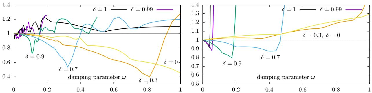
Figure 3: Convergence of the operator related damped Newton scheme for different damping parameters  $\delta$ . Each figure shows the relative change of the residual after one Newton step for different linesearch parameters.
